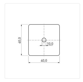
Height [mm]: 40 Inner Diameter [mm]: 10 Marking:
