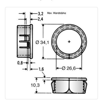
Color: Black Inner Diameter [mm]: 26.6 Material: PA 6.6 Plastic Material Group: Max. Panel Thickness [mm]: 3.2 Mounting Hole [mm]: 31.8 Outer Diameter [mm]: 34.1 Weight: 1.79g
