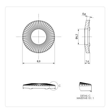
Finish: Plain For Thread Size: M4 Height [mm]: 8.0 Inner Diameter [mm]: 4.2
