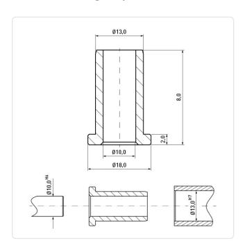
Color: Natural Flammability Class: UL94-V2 Inner Diameter [mm]: 10 Length [mm]: 8 Lug Diameter [mm]: 13
