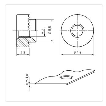
Finish: Plain Height [mm]: 2.8 Material: Steel Outer Diameter [mm]: 5.5 Panel Hole Ø [mm]: 4.2 Panel Thickness [mm]: 0,9 - 1,0 Thread Size: М3
