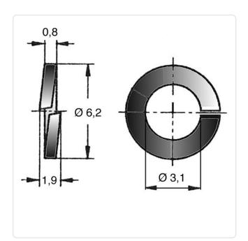
DIN/ISO: DIN127B Finish: Plain For Thread Size: M3 8.0 Height [mm]: Inner Diameter [mm]: 3.1
