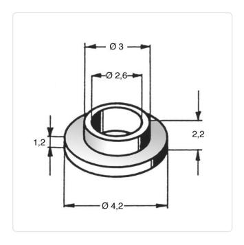
Color: Black Flammability Class: UL94-V0 2.2 Height [mm]: Inner Diameter [mm]: 2.6 Lug Diameter [mm]:
