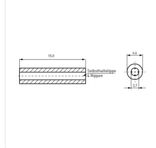
Color: Gray Flammability Class: UL94-V0 For Thread Size: M3 Inner Diameter [mm]: 3.7 Length [mm]: 15 Material: PVC - Polyvinyl Chloride Material Group: Plastic Outer Diameter [mm]: 6.4 Weight: 0.51g Conformities: Reach RoHS SVHC
