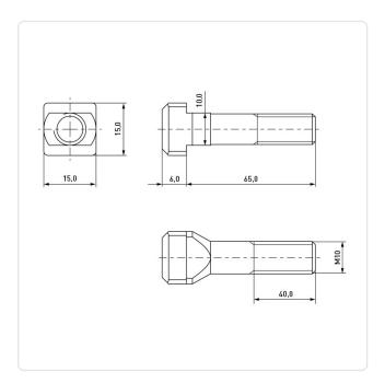
DIN/ISO: **DIN787** Plain Finish: Head Height [mm]:
