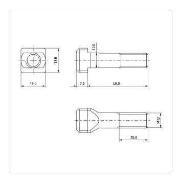
DIN/ISO: **DIN787** Finish: Plain Head Height [mm]:
