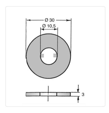
Color: Natural For Thread Size: M10 Height [mm]: Inner Diameter [mm]: 10.5 Material: PA 6.0 Material Group: Plastic Outer Diameter [mm]: 30 Weight: 1.95g
