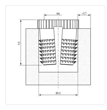
Finish: Plain Length [mm]: 9.5 Material: **Brass** Material Group: Brass Minimum Edge Distance [mm]: 2,7 Panel Hole Ø [mm]: 5.5 Thread Size: M4 Weight: 0.93g
