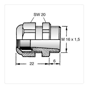
AF / OD [mm]: 20 Material: **Brass** Material Group: **Brass** Mounting Hole [mm]: 16.5 Panel Thickness Range [mm]: 5,0 - 10,0 Protection Code: **IP68** Thread Size: M16 Weight: 23.08g
