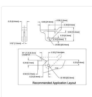
White Color: Flammability Class: UL94-V2 Material: PA 6.0 Material Group: **Plastic** Width [mm]: 6.35 Weight: 1.19g
