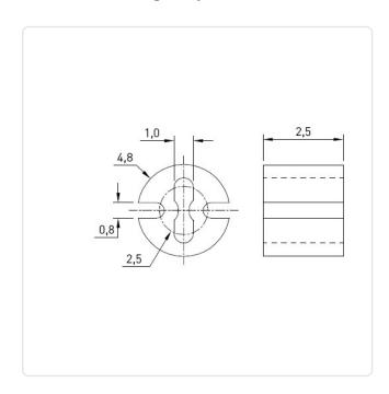
Color: Black Diameter [mm]: 4.8 Flammability Class: UL94-V0 LED Size [mm]: Ø3
