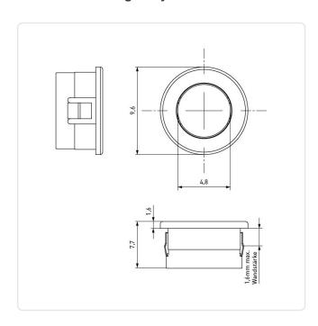
Color: Black Inner Diameter [mm]: 4.8 Material: PA 6.6 Material Group: Plastic Max. Panel Thickness [mm]: 1.6 Mounting Hole [mm]: 7.9 Outer Diameter [mm]: 9.5 Weight: 0.22g
