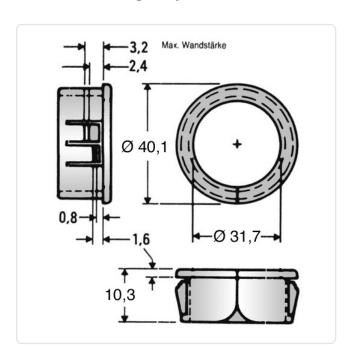
Color: Black Inner Diameter [mm]: 31.7 Material: PA 6.6 Plastic Material Group: Max. Panel Thickness [mm]: 3.2 Mounting Hole [mm]: 38.1 Outer Diameter [mm]: 40.1 Weight: 2.8g
