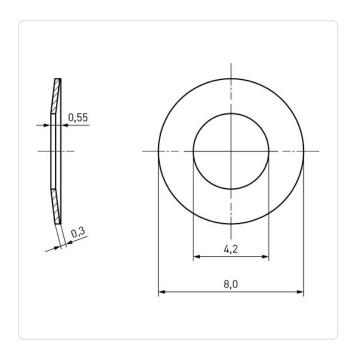
DIN/ISO: **DIN2093** Finish: Plain For Thread Size: M4 0.3 Height [mm]: Inner Diameter [mm]: 4.2
