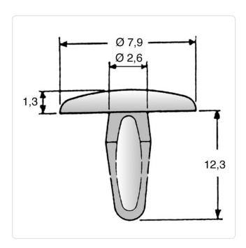
Color: Black Flammability Class: UL94-V2 Head Diameter [mm]: 7.9 Material: PA 6.6 Material Group: **Plastic** Mounting Hole [mm]: 2.7 Weight: 0.11g
