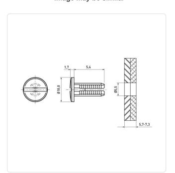
Color: Black Head Diameter [mm]: 10 Material: PA 6.6 Material Group: Plastic Mounting Hole [mm]: 5.5
