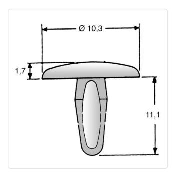
Color: Natural Flammability Class: UL94-V2 Head Diameter [mm]: 10.3 PA 6.6 Material: Material Group: **Plastic** Mounting Hole [mm]: 3.5
