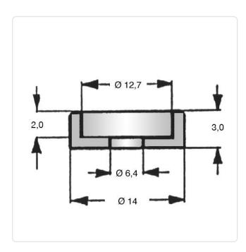
Color: Black For Thread Size: M6 Height [mm]: Inner Diameter [mm]: 6.4 Material: PA 6.0 Material Group: Plastic Outer Diameter [mm]: 14 Weight: 0.2g
