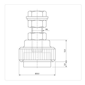
Diameter [mm]: 20 Height [mm]: 15 Material: Steel Thread Size: M6 Weight: 30.52g
