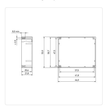
Color: Black Flammability Class: UL94-HB Height [mm]: 21.8 Length [mm]: 44 PA 6.0 Material:
