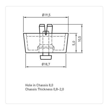
Color: Black Diameter [mm]: 19.5 Flammability Class: UL94-V0 Height [mm]: 10.4
