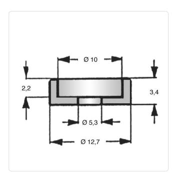
Color: Black For Thread Size: M5 Height [mm]: 3.4 Inner Diameter [mm]: 5.3 Material: PA 6.0 Material Group: Plastic Outer Diameter [mm]: 12.7 Weight: 0.26g
