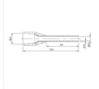
Color: Blue Finish: **Tin-Plated** Insulation: Polypropylene Length [mm]: 14 **Electrolytic Copper** Material: Material Group: **Electrolytic Copper** Plug-In Length [mm]: 8 Wire Cross Section [mm<sup>2</sup>]: 2.5 Weight: 0.15g Conformities:
