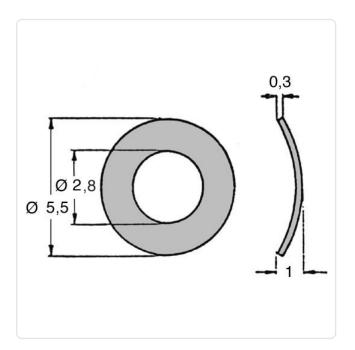
DIN/ISO: DIN137A Finish: Plain For Thread Size: M2.5 0.3 Height [mm]: Inner Diameter [mm]: 2.8
