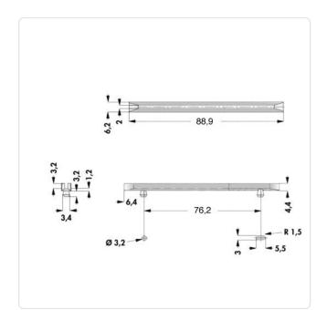
Color: Natural Dist. Mounting Holes [mm]: 76.2 Flammability Class: UL94-V2
