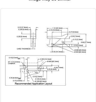
White Color: Flammability Class: UL94-V2 PA 6.0 Material: Material Group: **Plastic** 7.9 Width [mm]: Weight: 1.83g
