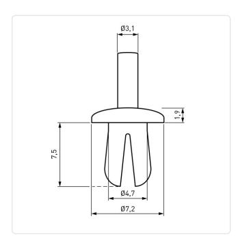
Color: Natural UL94-V2 Flammability Class: Head Diameter [mm]: 7.2 Head Height [mm]: 1.9 Length [mm]: 7.5 Mandrel Diameter [mm]: 3.1 PA 6.6 Material:
