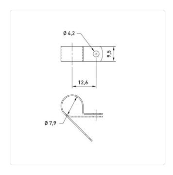
Bundle Diameter [mm]: 7,9 Natural Color: Distance Middle/Middle [mm]: 12.6 UL94-V2 Flammability Class: Material: PA 6.6 Material Group: Plastic Mounting Hole [mm]: 4.2 Thickness [mm]: 1.3 Width [mm]: 9.5
