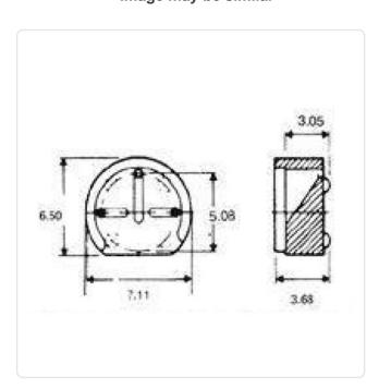
Color: Black Material: PA 6.0 Material Group: Plastic Model: TO-18 Outer Diameter [mm]: 7.1 Weight: 0.14g
