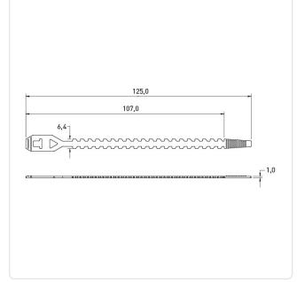
Bundle Diameter [mm]: 21,0-50,0 Color: Natural Length [mm]: 125 PE - Polyethylene Material: Material Group: Plastic **Ball Cable Tie** Model: Width [mm]: 6.4 Weight: 0.71g Conformities: Reach RoHS
