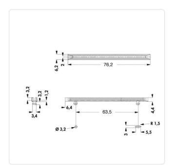
Color: Natural Dist. Mounting Holes [mm]: 63.5 Flammability Class: UL94-V2 Length [mm]: 76.2 PA 6.6 Material: Material Group: Plastic
