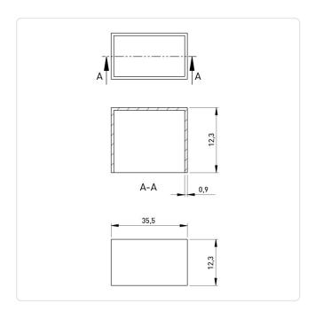
Color: Black Flammability Class: UL94-V0 Height [mm]: 12.3 35.5 Length [mm]:
