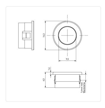
Color: Black Inner Diameter [mm]: 9.5 Material: PA 6.6 Material Group: Plastic Max. Panel Thickness [mm]: 1.6 Mounting Hole [mm]: 12.7 Outer Diameter [mm]: 14.3 Weight: 0.37g
