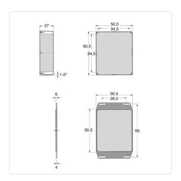
Height [mm]: 27 Length [mm]: 50.5 Material: Aluminum Material Group: Aluminum Protection Code: IP54 Width [mm]: 50.5
