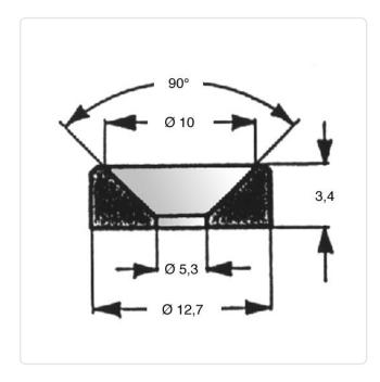
Color: White For Thread Size: M5 Height [mm]: 3.4 Inner Diameter [mm]: 5.3 Material: PA 6.0 Material Group: Plastic Outer Diameter [mm]: 12.7 Weight: 0.32gConformities:
