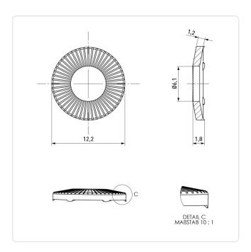
Finish: Plain For Thread Size: M6 Height [mm]: 1.2 Inner Diameter [mm]: 6.1
