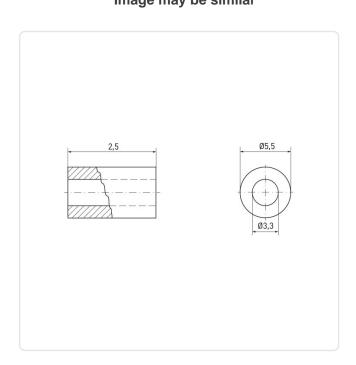
Finish: Plain For Thread Size: М3 Inner Diameter [mm]: 3.3 Length [mm]: 2.5
