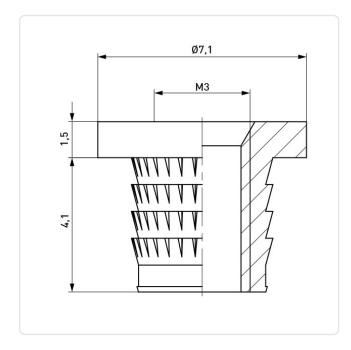
Finish: Plain Head Diameter [mm]: 7.1 Length [mm]: 4.1 Material: Brass Material Group: Brass Minimum Edge Distance [mm]: 1.7 Panel Hole Ø [mm]: 4 Thread Size: М3 Weight: 0.6g
