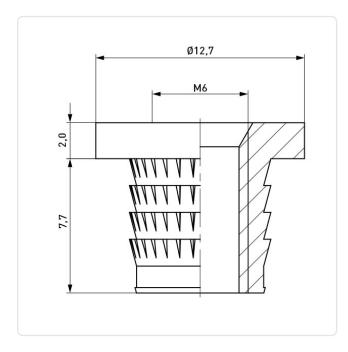
Finish: Plain Head Diameter [mm]: 12.7 Length [mm]: 7.7 Material: **Brass** Material Group: Brass Minimum Edge Distance [mm]: 3.3 Panel Hole Ø [mm]: 8 Thread Size: M6 Weight: 3.23g
