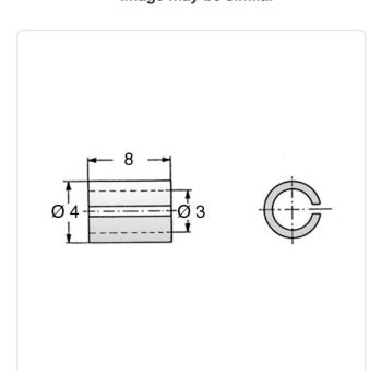
Height [mm]: 8 Inner Diameter [mm]: 3 Material: **Brass** Material Group: **Brass**
