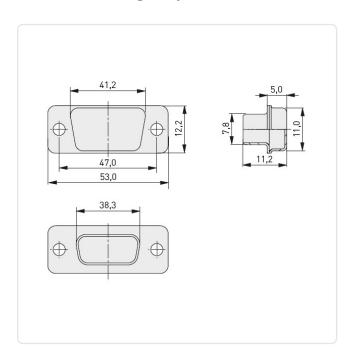
Material: Steel Steel Material Group: Model: D-Sub Mounting Hole [mm]: 3.2 Width [mm]: 53 Weight: 5.4g
