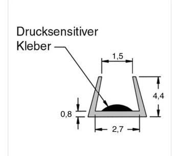
Application Thickn. [mm]: 2.7 Color: Natural Flammability Class: UL94-HB
