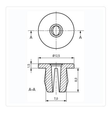
AF / OD [mm]: 12.5 Color: Black Head Height [mm]: 1.5 Length [mm]: 8 PA 6.6 Material: Material Group: **Plastic** Panel Cutout [mm]: 7.0x7.0 Panel Thickness [mm]: 0,8-4,0 Thread Diameter [mm]: Ø 4.2 Weight: 0.45g Conformities:
