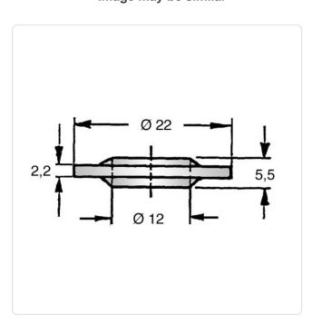
For Thread Size: M12 5.5 Height [mm]: Inner Diameter [mm]: 12.2 Material: PA 6.0 Material Group: Plastic Outer Diameter [mm]: 22 Weight: 0.46g
