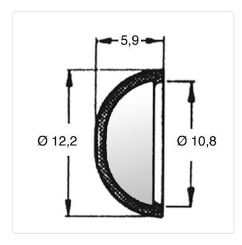
Color: Gray Head Height [mm]: 5.9 Inner Diameter [mm]: 10.8 PA 6.0 Material: Material Group: **Plastic**
