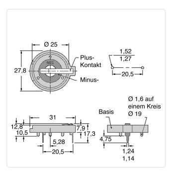
Battery Type: Cell Dia. 24mm
